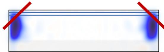
Figure 2.15: Schematic of a  $3\mu\text{m}$  diameter disk with truncated edges and depicting the  $H_z$  field of a first order radial mode.
