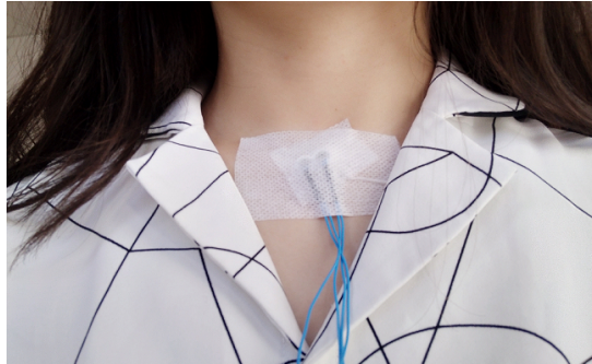
Figure 2.2: Position of the microphones: two microphones are inserted into the support that is fixed at suprasternal notch with two strips of adhesive tape.
