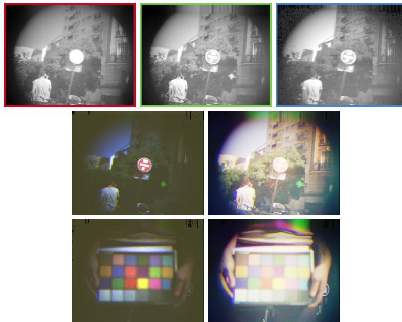
Fig. III.7 The figure’s top row shows reconstructed frames from events acquired by each sensor of the three-chip event-based camera. The grey levels are tone-mapped with a logarithmic function in order to be displayed on a regular screen. The bottom-left frames are reconstructed with the linear color model presented in the methodology. The colors are properly reconstructed, but very little detail is left in dark areas. The bottom-right frames use the channels’ logarithmic tone-mappings as their color channel, yielding incorrect colors but much more details in dark areas.
