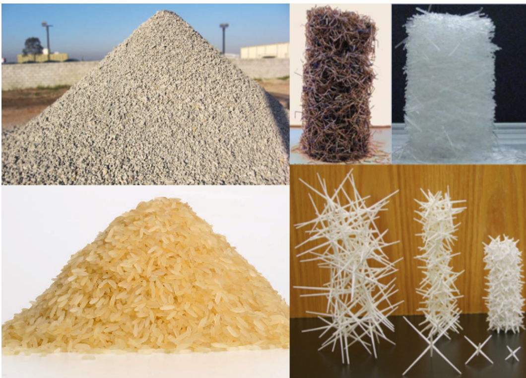
Figure 1.14 – On the left column, heaps of rather spherical particles – photos taken from the internet. On the right, column-like stacks of staples, rods and stars, photos taken from [121, 122, 49].
