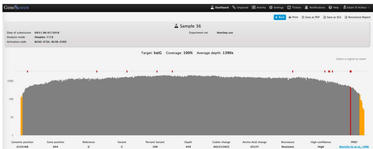
Figure 19: Individual target view mode, showing detailed sequencing data obtained for the katG gene in a sample. Coverage breadth (i.e. the fraction of the reference covered by a minimum of 5 reads) and the average coverage depth are shown at the top. Red boxes on the dotted line indicate known positions of resistance mutations included in the built-in reference databases. Orange and grey zones in the histogram indicate coverage depths below and above 200 x (note that the scale on the right is logarithmic). The bottom part shows detailed information for the position in which a drug resistance associated S315T mutation was detected in the sample.
