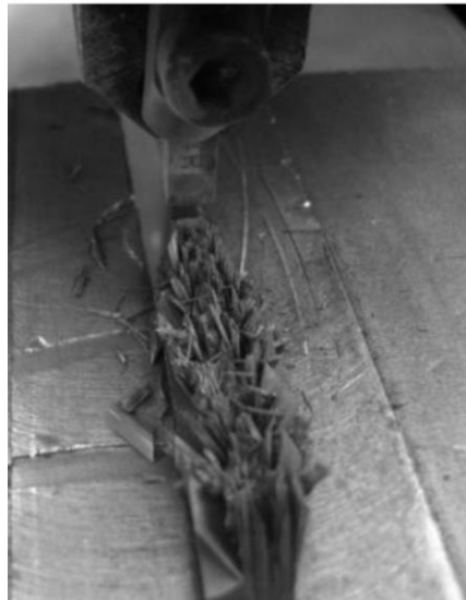
Fig. 1.1.19: Damage to specimens with tool H13A ( X_2 = 1350 ) [Iliescu, 2008].
