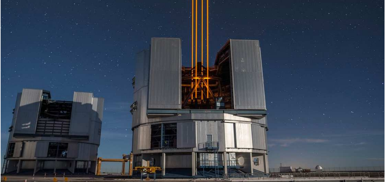
Figure 2.2: UT4 telescope on which MUSE is mounted, with the four adaptive optics lasers in action.
