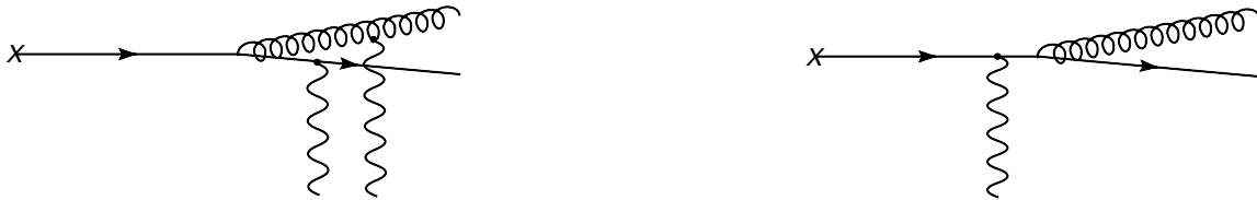
Figure 2.1: Soft gluon coherence: the sum of the diagrams in which the soft gluon (waved line) is emitted from any of the external partons (left diagram) is equivalent to the diagram where the soft gluon is emitted strictly before the hard gluon (right diagram). The figure is taken from [35].
