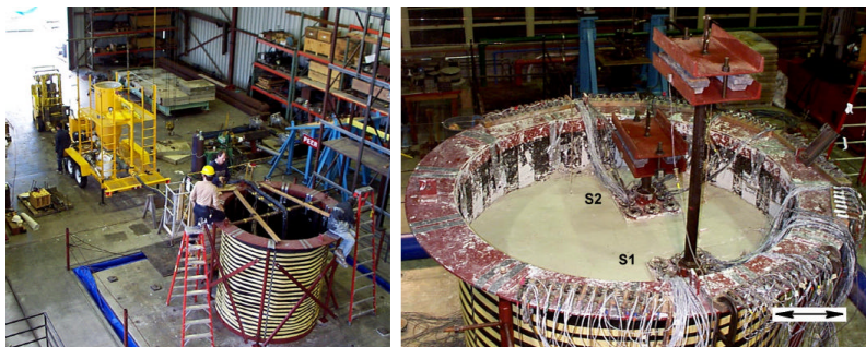
Figure 2.19: Shaking table tests, full scale container mounted on the shaking table to study the seismic interaction of soft clay-pile-superstructure, Meymand [143]
