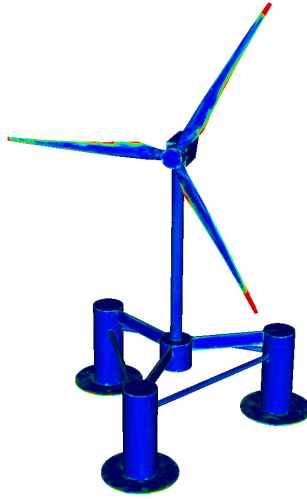
Figure 2.20: Distance e_{AB} with A mesh representing the immersed FOWT and B iso-surface \Phi_\varepsilon = 0 with \varepsilon = 5 \cdot 10^{-2}m . Plot of the distance scaling from 0 to 10^{-2}m .
