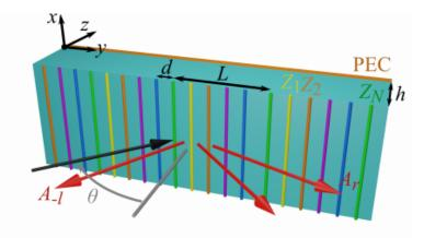
Figure 2.1: System under consideration: a periodic array of thin loaded wires (represented by color cylinders) placed on a PEC-backed dielectric substrate having relative permittivity  $\varepsilon_s$ , permeability  $\mu_s$  and thickness h. The array is excited by a plane wave incident at the angle  $\theta$  (black arrow). Propagating diffraction orders are illustrated by red arrows.
