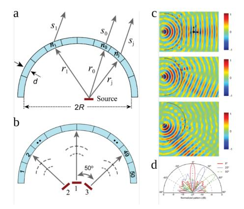
Figure 1.16: (a), (b) The principle of beam-steering with a semi-cylindrical metasurface antenna when being illuminated by a single feeding antenna (a) or multiple feeding antennas (b). (c), (d) Results of 2D simulations of a semi-cylindrical metasurface. The panel (c) demonstrates distributions of the electric field for beam-steering at  $0^{\circ}$ ,  $25^{\circ}$  and  $50^{\circ}$ . The panel (d) shows corresponding far-field radiation patterns [100].
