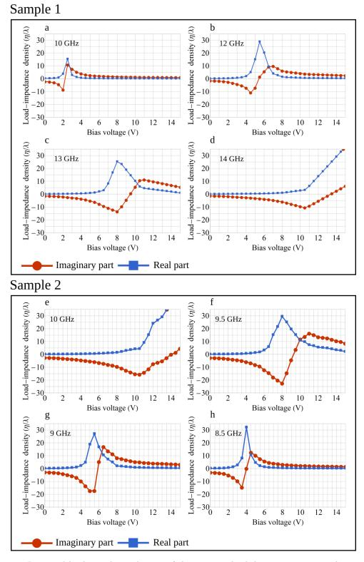
Figure 5.10: Retrieved load-impedance density of the varactor-loaded wire constituting the sparse metasurface vs. the bias voltage. The panels show examples at different frequencies indicated in top right corner. It is seen how the position of the resonance shifts when the frequency is changed. The panels (a)-(d) and (e)-(h) correspond to the sample 1, Fig. 5.7(c), and the sample 2, Fig. 5.7(d), respectively.
