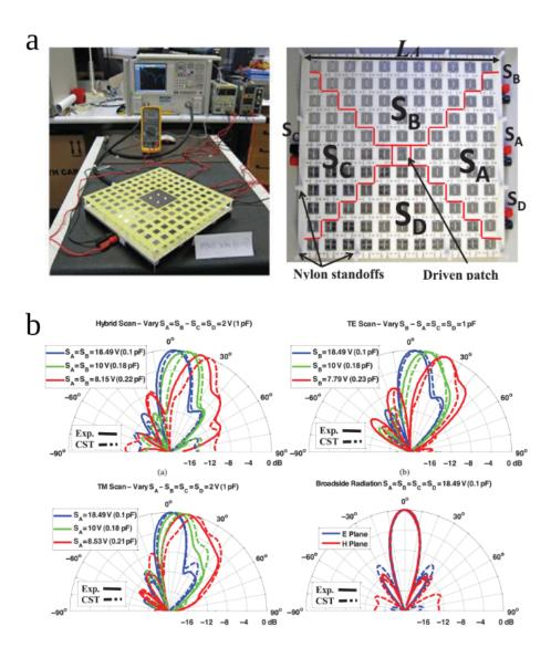
Figure 1.15: (a) Photographs of the assembled antenna prototype (left) and the reconfigurable metasurface (right). (b) Simulation and experimental results of normalized radiation patterns at 5. GHz operating frequency for different azimuth and elevation steering angles [99].
