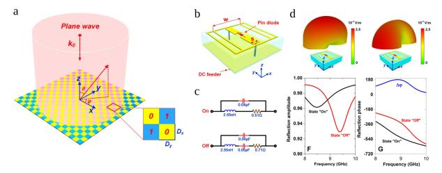
Figure 1.1: (a) An illustration of a binary phase-state metasurface illuminated by a normally incident plane wave. (b) A schematics of a unit cell loaded with a PIN diode. (c) A circuit model of a PIN diode in ON and OFF states. (d) Radiation patterns and the local reflection coefficient from a binary phase-state unit cell [76].
