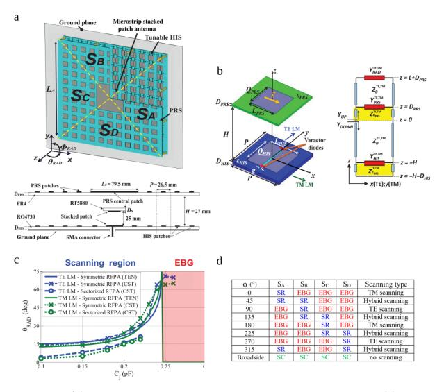
Figure 1.14: (a) A schematic of a metasurface-based reconfigurable Fabry-Perot antenna. (b) A layout of a unit cell design (left) and the transverse equivalent network for TE- and TM-polarized leaky-waves. (c) Elevation scanning angle vs. the capacitance of varactor diodes at 5.5 GHz operating frequency. (d) The table shows azimuth scanning angle as function of activated sectors of the reconfigurable metasurface [99].
