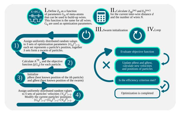
Figure 3.3: A block diagram of a particle swarm optimization algorithm.
