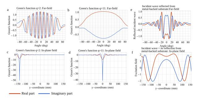
Figure 5.3: (a)–(d) Examples of the Green's function calculated for the positions of  $2^{nd}$  and  $11^{th}$  wires in the far-field (a), (b) and in the plane of wires (c), (d). (e) The normally incident cylindrical wave reflected from the PEC-backed dielectric substrate in the far-field. (f) The excitation field (incident wave plus its reflection from the PEC-backed substrate) in the plane of wires.
