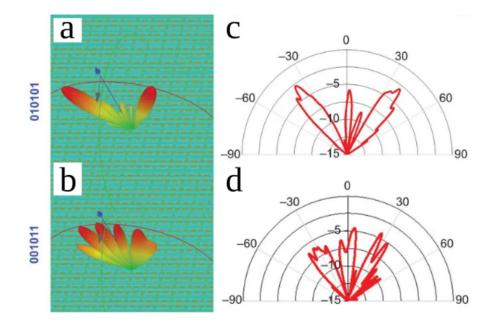
Figure 1.7: Simulation (a), (b) and experimental (c), (d) results of excitation of multiple beams with the reconfigurable binary phase-state metasurface. The operating frequency is 8.6 GHz [37].
