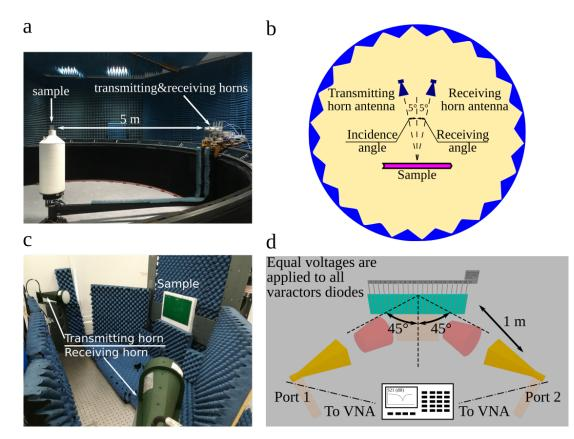
Figure 5.8: Photographs (a), (c) and schematics (b), (d) of the experimental setups used to characterize sample 1 (a), (b) and sample 2 (c), (d).
