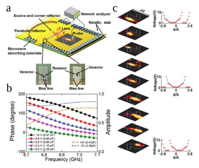
Figure 1.19: (a) A schematic of the experimental setup. The inset figure shows photographs of the fabricated unit cell, frontside (right) and backside (left). (b) The phase and the amplitude of the local transmission coefficient under different applied bias voltages (c) Experimental results of the near-field scanning at 6.9 GHz, the focal spot is consequently moved along a trace of the letter "N" [47].
