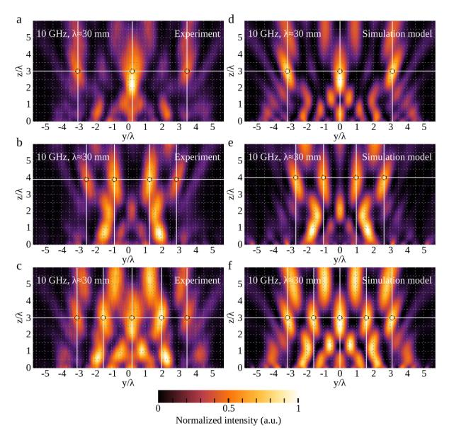
Figure 5.19: Different examples of creating three (a), four (b) and five (c) focal spots at 10 GHz. The panels (a)-(c) and (d)-(e) show experimental and corresponding simulation results, respectively.
