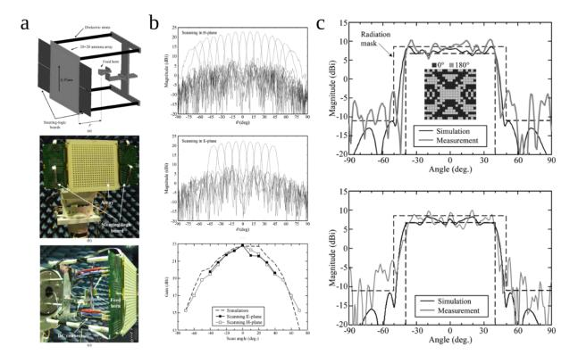
Figure 1.5: (a) A schematic and photographs of the assembled experimental sample. (b) Experimental results of beam steering in H-plane (top) and E-plane (central). The bottom panel compares measured and simulated gain of the sample. (c) Experimental results of beam-shaping. The top and bottom panels correspond to H- and E-planes, respectively. The operating frequency is 9.8 GHz [35].
