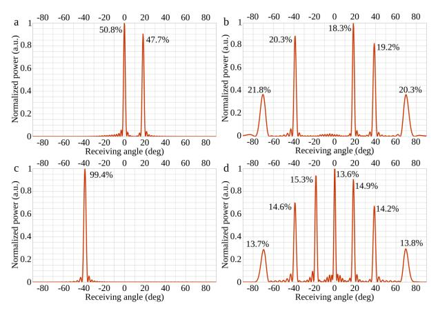
Figure 2.3: (a)-(d) Period  $L = 3 \times 30/(\sin(70^{\circ}))$ , there are seven propagating diffraction orders. (a)  $0^{\text{th}}$  and  $1^{\text{st}}$  orders are excited. (b) All orders are excited apart from  $0^{\text{th}}$  and  $-1^{\text{st}}$ . (c) only  $-2^{\text{nd}}$  order is excited. (d) All propagating orders are excited.
