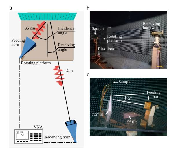
Figure 5.11: A schematic illustration (a) and photographs (b), (c) of the experimental setup to measure far-field radiation patterns.
