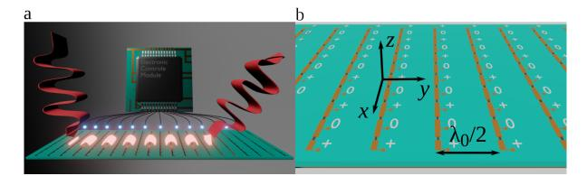
Figure 5.1: (a) An illustration of a strongly non-local reconfigurable sparse metasurface converting a normally incident wave into an anomalously reflected wave via an excited surface wave. The surface wave propagates long the metasurface and manifests its strongly non-local response. The electronic control module represents a multichannel DC voltage source run by a Raspbery Pi nano-computer. (b) A close-up of a region of the sparse metasurface.
