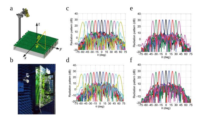
Figure 1.3: (a), (b) A schematic of the assembled experimental sample (a) and its photograph in an anechoic chamber (b). (c)–(f) Experimental results of beam-steering in different planes and at different frequencies. The panels (c) and (d) correspond to x0z and y0z planes, respectively, the operating frequency is 11.1 GHz. The panels (e) and (f) correspond to x0z and y0z planes, respectively, the operating frequency is 14.3 GHz [79].
