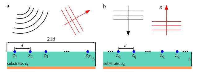
Figure 5.4: (a) A sparse metasurface demonstrating an anomalous reflection when being illuminated by a cylindrical wave. The sparse metasurface is represented by a **finite** array of wires having different load-impedance densities  $Z_q$ . (b) A periodic array of wires having all the same load-impedance density  $Z_q$ . The array is illuminated by a normally incident plane wave and the reflection coefficient R is calculated by means of Eqs. (3.1) and (3.4).
