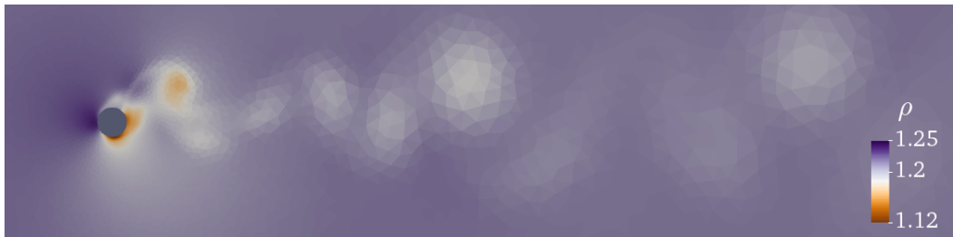
Figure 4.8 Instantaneous density field of a flow around a vertically oscillating cylinder at Re = 185 , A_e = 0.5 and f_r = 1.2 .
