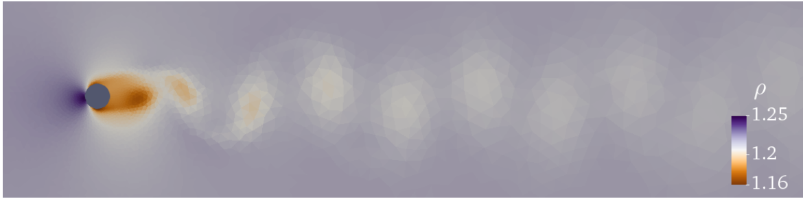
Figure 4.2 Instantaneous density field of a flow around a vertically oscillating cylinder at Re = 185 , A_e = 0.2 and f_r = 0.8 .
