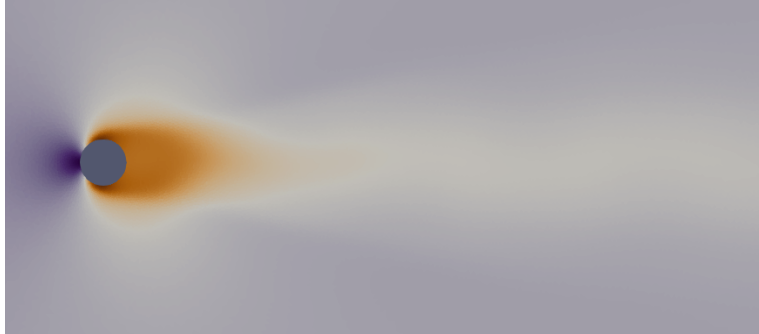
Figure 3.5 First proper orthogonal mode (POM of density) for the flow around a fixed cylinder at Re = 100 .
