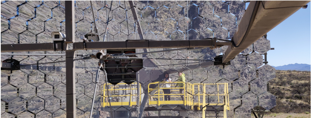
Fig. 3.8. — T1 view from the focal plane taken by the author. The camera, with the shutter closed, can be seen reflected in the mirrors. The sky and reflectivity cameras are located on the reflector, close to the center where there are no mirrors. The LED flasher is also mounted on the crossbeam. In the picture, the shifters on call start preparing for observations.
