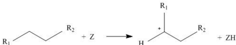
Figure 6: Hydride abstraction - formation of an alkylcarbenium ion
