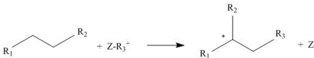
Figure 9: Oligomerization - formation of larger alkylcarbenium ions
