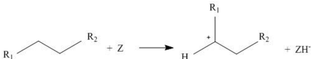
Figure 6: Hydride abstraction - formation of an alkylcarbenium ion
