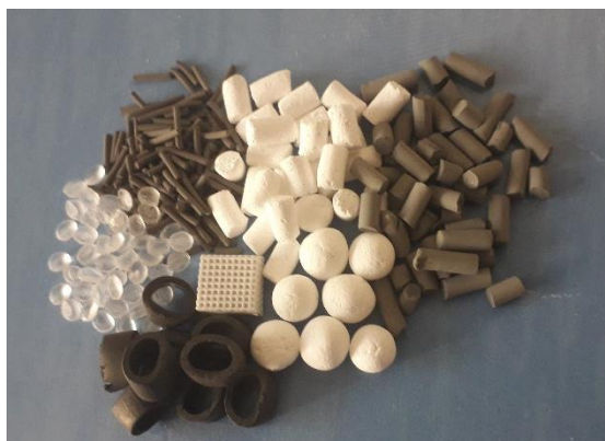
Figure 15: Different industrial catalysts morphologies
