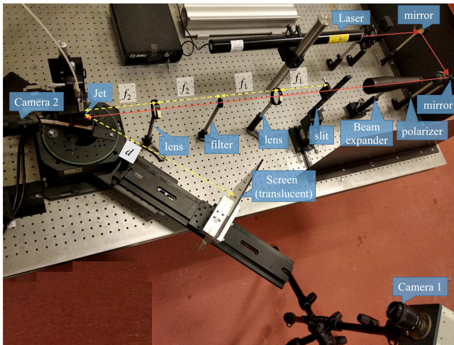
Fig 5.9 Experimental setup for measuring the scattered intensity by a liquid jet.
