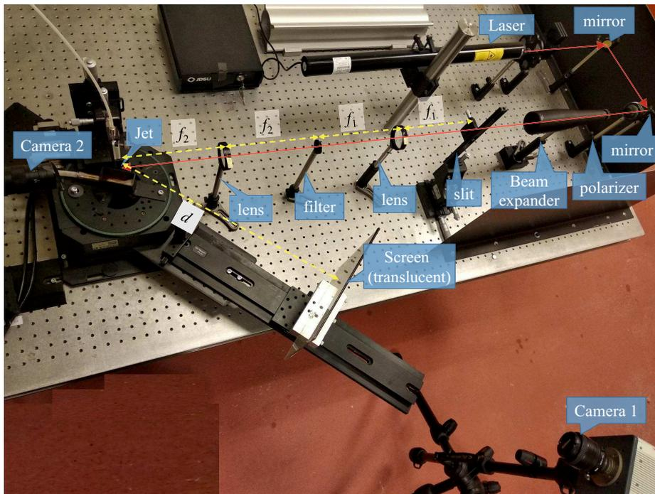
Fig 5.9 Experimental setup for measuring the scattered intensity by a liquid jet.
