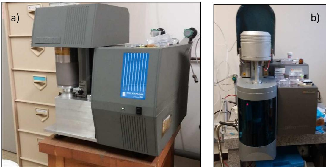
Figure 31: Thermobalances : a) Labsys b) Setsys
