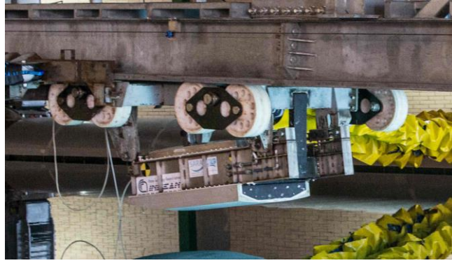
FIGURE 5.2: The trolley is attached to the guide. It carries the acquisition box and the tested specimen [44].
