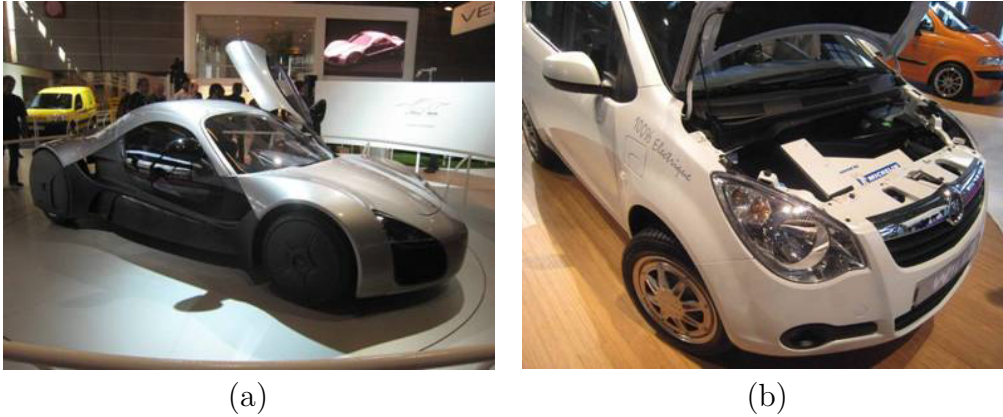
Figure 1.18. Light electric vehicles equipped with Active Wheel: (a) Venturi Volage, (b) Heuliez Will.
