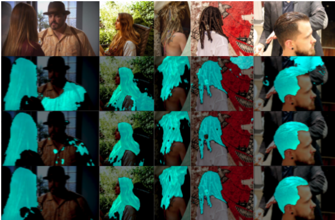
FIGURE 6.4: Comparison on challenging examples in Figaro1k. First row: Input image. Second row: Segmentation results by our model without detection stage. Third row: Segmentation results by ImageNet pre-trained DeepLabV3+. Fourth row: Segmentation results by our two-stage model. Many tiny isolated false positives can still be observed on the man’s shirt in the first image of DeepLabV3+ results.
