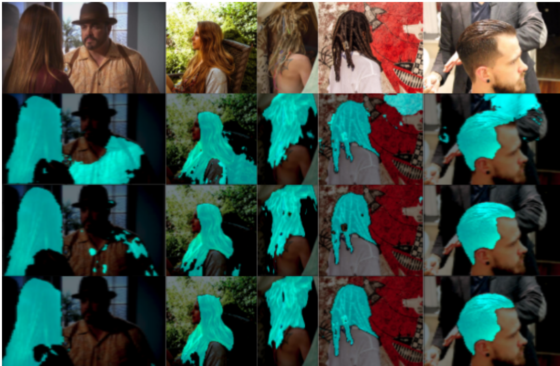
FIGURE 6.4: Comparison on challenging examples in Figaro1k. First row: Input image. Second row: Segmentation results by our model without detection stage. Third row: Segmentation results by ImageNet pre-trained DeepLabV3+. Fourth row: Segmentation results by our two-stage model. Many tiny isolated false positives can still be observed on the man’s shirt in the first image of DeepLabV3+ results.
