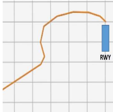
(b) A more precise view of a portion of the route. The turns are made as the discretization allows. The maximum turn angle constraint is met.
