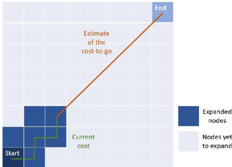
Figure 2.13 – An illustration of the principle of the A^* algorithm.
