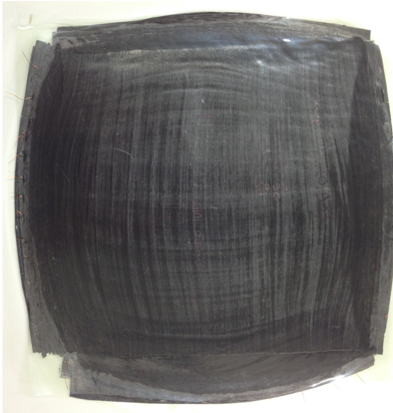
Figure 1.5 – Photograph of the [0/90]_6 sample after compression.
