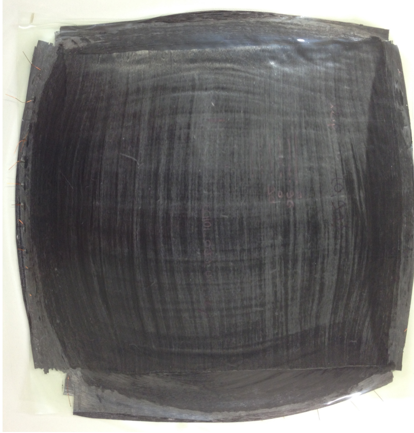
Figure 1.5 – Photograph of the [0/90]_6 sample after compression.
