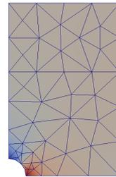
Figure 6.18: Thermal adapted mesh obtained using Rivara's technique.
