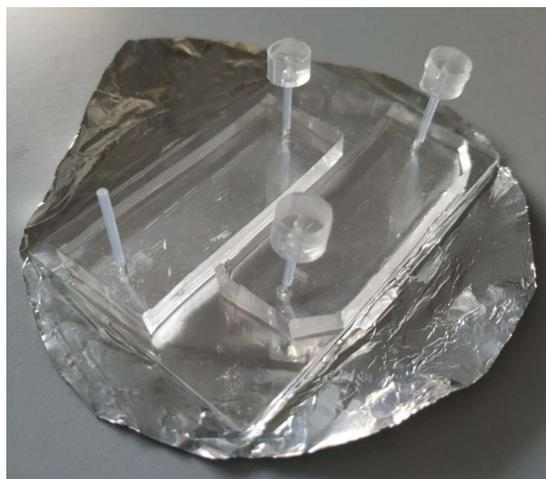
***Figure A.1.*** Two chips of a pulsation dampener on a glass slide. The tubing is already plugged into the chip and custom-made PDMS connection are placed on 3 of them. The tubing on the left side is left unconnected for clarity.
