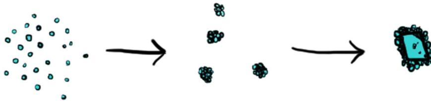
**Figure 3.51.** *Particles nucleating and growing through an aggregation mechanism.*
