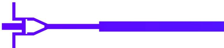
**Figure 3.7.** Geometry of the nozzle and exit channel in the *Purple Chip A*.
