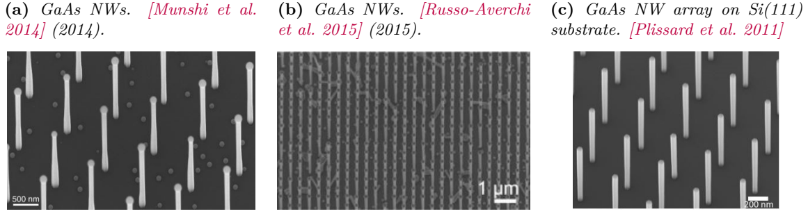
Figure 3.5: Examples of self-catalyzed GaAs NW arrays on silicon using MBE.
