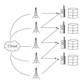
Figure 7.1: The Wyner's network where each transmitter is connected, via an individual link, to the backhaul from where it can fetch  $M_T \cdot f$  bits. Each user is equipped with a cache of normalized size  $\gamma$ . Receiver k + 1 can only receive messages from transmitters k and k + 1.
