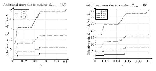
Figure 3.1: Maximum achievable effective caching gain  $\bar{G}_L = D_L(K, \gamma) - L$ (maximized over all possible K), achieved by the new scheme for different L, under subpacketization constraint  $S_{\text{max}} = 3.6 \cdot 10^4$  (left) and  $S_{\text{max}} = 10^6$  (right).
