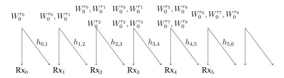
Figure 7.9: One transmission slot in the non-cache-aided network with backhaul constraint of  $M_T = \frac{5}{2}$  corresponding to Eq. (7.5). This slot involves a subnetwork of 9 users and delivers 8 packets (to all users apart from the 4<sup>th</sup>), thus achieving a pudDoF of  $d\left(\frac{5}{2},0\right) = \frac{8}{9}$ .
