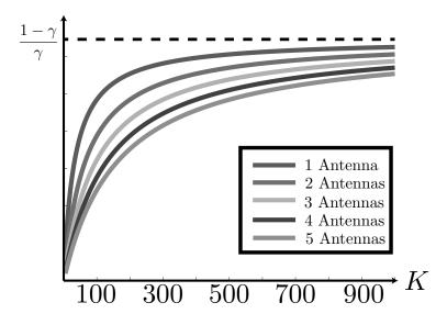
Figure 2.1: The delivery time as a function of the number of users K for various values of transmit antennas, as is theoretically achieved by the Coded Caching scheme of [1] and the multi-antenna schemes [10, 11] for a fixed normalized cache per user of fraction  $\gamma$ . We can see that the effect of introducing antennas to the system can only marginally improve the delay, and as users keep growing then this delay approaches the lower bound delay of  $T_b = \frac{1-\gamma}{\gamma}$ .
