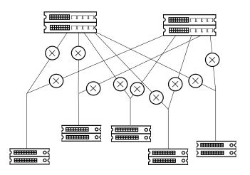
Figure 8.1: Illustration of the wired setting.  $\times$  denotes a network coding operation.
