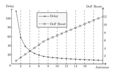
Figure 9.3: The improvement in the delay and the DoF boost that are achieved as a function of the number of antennas for a scenario with  $K_1 = 100$  cacheaided users with normalized cache-size  $\gamma_1 = \frac{1}{20}$  and  $K_2 = 120$  cache-less users. We can see that the DoF boost slope becomes smaller after L = 7 antennas, showing that any cache-size unevenness effect has been completely removed, thus the DoF continues to increase additively instead of multiplicatively.
