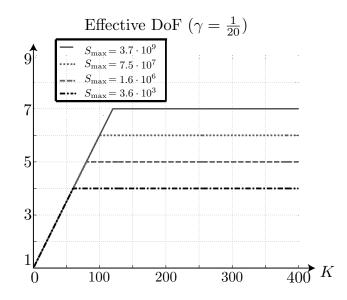
Figure 2.2: Maximum effective DoF  $\overline{D}_1$  achieved by the original centralized algorithm (single antenna,  $\gamma = \frac{1}{20}$ ) in the presence of different subpacketization constraints  $S_{\text{max}}$ . The gain is hard-bounded irrespective of the number of users K (x-axis).
