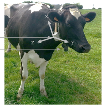
Fig. 2. RF-Track 3D accelerometer and GPS sensor fixed on the collar on the cow. The three coordinate axes of the accelerometer sensor are displayed.
