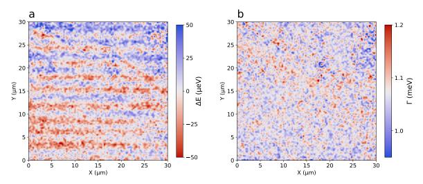
Figure 3.28 Spatial variations of the shift  $\Delta E$  (a) and broadening  $\Gamma$  (b) of the Raman-active mode of hBN at  $1370\,\mathrm{cm}^{-1}$  (170 meV) in a  $30\times30~\mathrm{\mu m}^2$  region of sample C40 at 10 K. The average Raman-mode energy is 169.78 meV.
