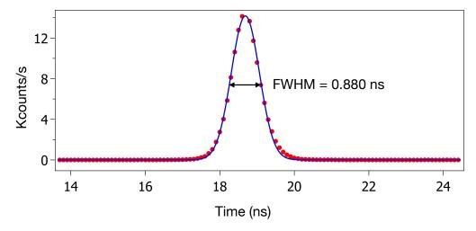
Figure 2.8 Instrument response function (IRF) of the detection setup. 50 ps laser pulses are sent to probe the temporal broadening induced by the electronics of the detectors. Red circle are data whereas the solid blue line is a gaussian fit to the data. FWHM = 880 ps.
