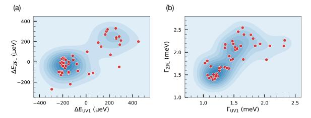
Figure 3.23 (a) Correlation plot of the shifts  $\Delta E$  of the UV1 line and ZPL of the 4.1 eV defect. The average UV1 energy is 4.1197 eV, and the average ZPL energy is 4.0974 eV. (b) Correlation plot of the widths  $\Gamma$  of the same peaks as in (a).
