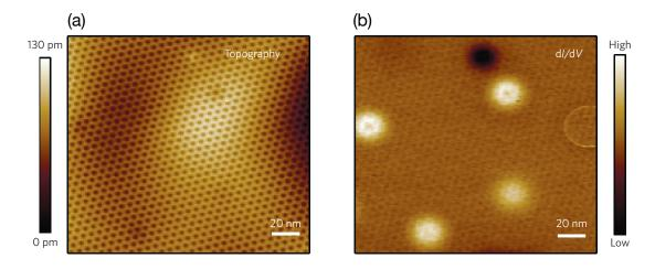
Figure 1.20 STM topography (a) and corresponding dI/dV map (b) for a single layer of graphene deposited on top of a BN crystal. On (b) can be seen bright and dark dots as well as a ring  $\sqrt{75}$ .
