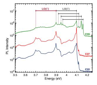
Figure 3.7 Full set of the PL spectra (semilog scale) of carbon-doped hBN samples in the 3.5-4.25 eV range. The spectra are vertically shifted for clarity. The horizontal bars have a 200 meV width, corresponding to the  $LO(\Gamma)$  phonon energy.
