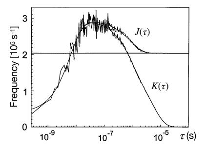
Figure 2.9 Histograms  $K(\tau)$  and  $J(\tau)$ . The wiggly  $K(\tau)$  is the normalized histogram of the experimental interphoton times measured on a molecule. The wiggly  $J(\tau)$  was calculated using FFT. The smooth  $J(\tau)$  is a fit and the smooth  $K(\tau)$  is the corresponding prediction 107.
