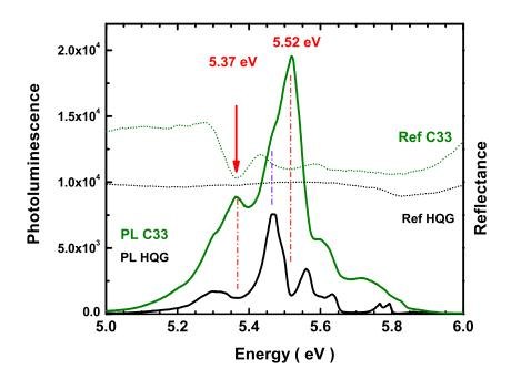
Figure 3.6 PL (solid lines) and reflectance (dotted lines) spectra on linear scales, recorded in a test undoped hBN crystal (HQG, black lines) and a heavily carbon-doped one (C33, green lines) at 10 K. Note the coincidences between the reflectance minima and the PL maxima in sample C33.
