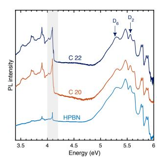
**Figure 3.3**Macro-PL spectrum at 8 K (semilog scale), with an excitation energy of 6.35 eV, in bulk hBN synthesized either with iron (C22) or nickel (C20), and the hBN powder used as a precursor, here in the form of HPBN.
