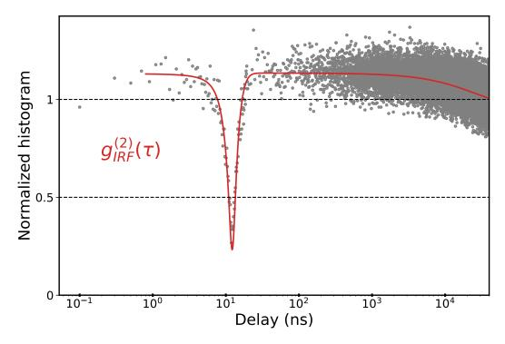
Figure B.2  $g^{(2)}(\tau)$  curve fitting using Eq (B.17) with taking the IRF of the detection setup into account. Grey circle are experimental data and red solid line is the fit.
