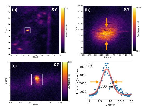
Figure 3.32 XY PL scan on a flake (a) and a zoom on the bright spot indicated by the square (b) complemented by a XZ scan in depth (c). Temperature is 4 K, excitation power 0.3 mW. (d) Intensity profile of the vertical cross-section on (b) at  $X = 6.5 \, \mu m$ .
