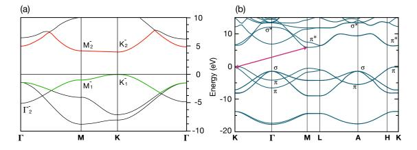
Figure 1.10 Calculated electronic band structure of 2D [46] (a) and 3D [47] (b) hBN. The electronic gap is direct in 2D at the K point of the Brillouin zone, while in 3D it is indirect with an upward transition from K to M.
