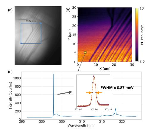
Figure 3.18 (a) Widefield image of a region of the hBN crystal. The blue square indicates a region of  $30\times30~\mu\text{m}^2$  on which is performed the SPIM acquisition (b). (c) is the spectrum extracted from the yellow pixel on (b). Inset: zoom on the ZPL of the emission and Gaussian fit (orange dotted line).
