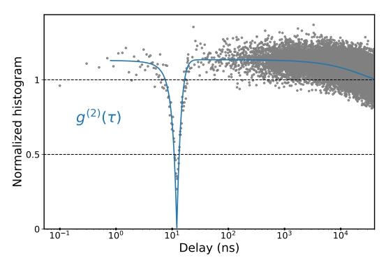
Figure B.1  $g^{(2)}(\tau)$  curve fitting using Eq (B.1) without taking the IRF of the detection setup into account. Grey circle are experimental data and blue solid line is the fit.
