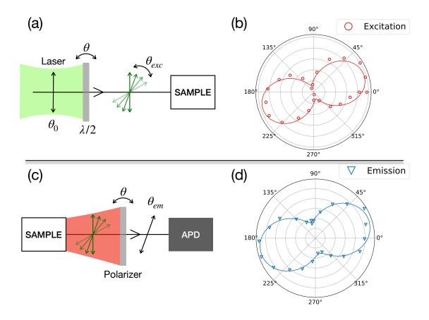
Figure 2.4 Schematic of the setup to perform excitation (a) and emission (c) polarization measurement, and corresponding angular diagrams for the excitation (b) and emission (d). The markers correspond to the data while the solid lines are fitting with a  $\cos^2(\theta)$  function.
