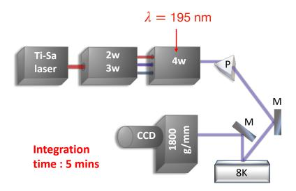
Figure 3.1 Scheme of the macro-photoluminescence setup. A Ti:Sa oscillator is quadrupled through two successive wave-mixing units, and sent onto the sample inside the cryostat. An achromatic optical system couples the emitted light to a spectrometer equipped with a camera optimized for deep UV.
