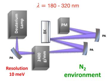
Figure 3.2 Scheme of the reflectivity setup. A deuterium lamp is spectrally filtered through a monochromator and sent onto the sample with near normal incidence angle. The intensity of the reflected field is measured with a photomultiplier.
