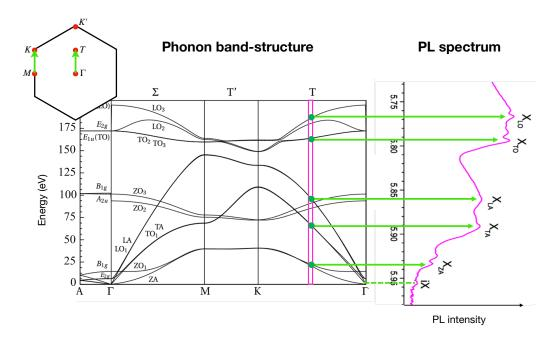
Figure 1.12 Photoluminescence spectra of BN (right side) plotted at the same scale as the phonon dispersion relation (left side) [56]. The energy of the photoluminescence line iX at 5.955 eV coincides with the zero phonon-energy.
