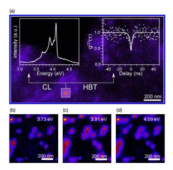
Figure 1.17 Cathodoluminescence spectrum of chemically exfoliated hBN flake suspended on a TEM grid (a-left) and normalized second-order correlation function (a-right) recorded on the emission spot in the white dotted square. (b,c,d) CL intensity maps of the peaks at 3.73, 3.91, and 4.09 eV, showing a perfect spatial match and therefore a unique origin 67.
