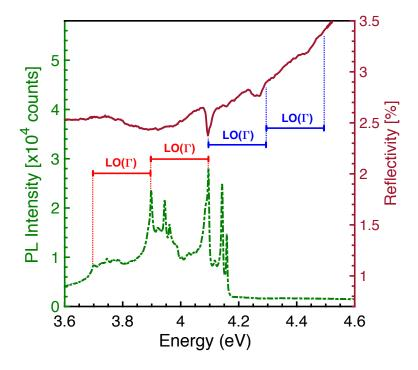
Figure 3.9 PL (green dashed line) and reflectivity (purple solid line) spectrum on linear scales, recorded at 8 K for sample C33 in the 4 eV region. The horizontal bars have a 200 meV width, corresponding to the LO( $\Gamma$ ) phonon energy. They are displayed in red for the red-shifted phonon-assisted emission (below 4.1 eV), and in blue for the blue-shifted phonon-assisted absorption (above 4.1 eV).
