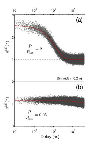
Figure 2.12 Second-order correlation function  $g^{(2)}(\tau)$  recorded for  $P/P_{sat} = 0.05$  (a) and  $P/P_{sat} = 2$  (b), for very long time delays and a bin width of the histogram of 0.2 ns. The data (black dots) are fitted using the full convoluted function of Eq. (2.22) (red solid lines).
