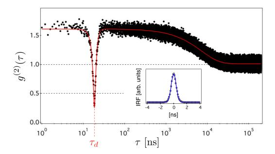
Figure 2.10  $g^{(2)}(\tau)$  function recorded from a PL spot for a laser excitation power  $P=150\,\mu\mathrm{W}$  and a bin width w=200 ps and displayed on a log x-scale. Black dots are experimental data and the solid red line is data fitting using a three-level model while including the IRF of the detection setup, see next section.  $\tau_d\approx 20$  ns is the electronic delay.
