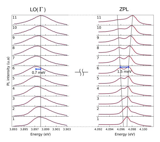
Figure 3.21 Series of spectra recorded at 200 nm from each other. The horizontal energy range selects only the ZPL (right) and its phonon replica  $LO(\Gamma)$  (left). The horizontal blue bars at the spectrum 6 indicates energy splitting of 1.5 meV between the two ZPL and an energy shift of 0.7 meV for the phonon replica. Gray lines are guidelines for the eyes.
