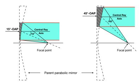
**Figure 3.16**Drawing of 15° and 45° off-axis parabolic mirrors (OAP). Parabolic mirrors are free of spherical aberrations.
