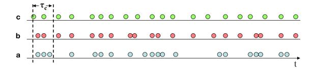
Figure A.1 Illustration of the different statistics of emission for a source.  $\tau_c$  represents a typical interval to evaluate the photon emission fluctuation. (a), (b), (c) represent the bunched type, coherent type and anti-bunched type, respectively.
