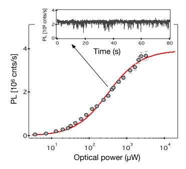
Figure 2.15 PL saturation curve of the defect. Inset: PL time trace recorded for a laser excitation power  $P=400~\mu\mathrm{W}$  performed on the same individual defect. The solid red line is the fit proposed in the main text. The dashed blue line shows the intensity at saturation for the NV center in diamond. The inset shows the stability of the emission at around 0.5 mW.
