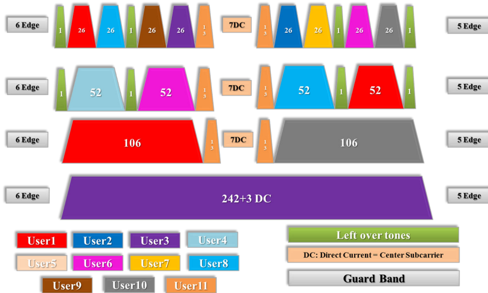
Figure 1.17: OFDMA configurations in 802.11ax for 20 MHz
