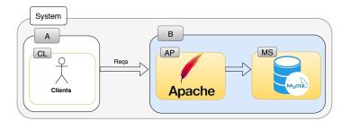
Figure 5.4 – Illustration of a Web stack comprising a pair of interacting components A and B, where B is a complex component composed of Apache server and MySQL database.
