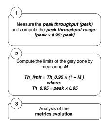
Figure 3.13 – Main steps of the analytical study for one given setup.
