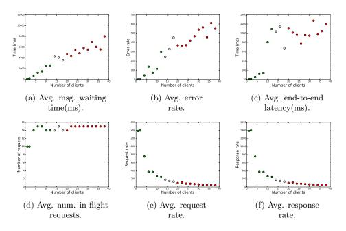
Figure 3.17 – Evolution of client software level metrics for setup-0 in the Kafka cluster use case.
