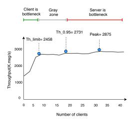
Figure 3.29 – Bottleneck identification for setup-0 of the Kafka/Spark cluster.
