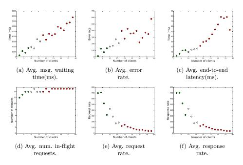
Figure 3.30 – Evolution of client software level metrics for setup-0 of the Kafka/Spark use case.
