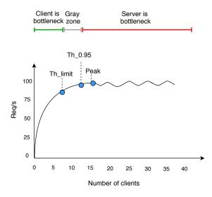
Figure 3.7 – Illustration of bottleneck identification based on throughput measurement.
