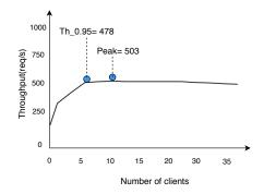
Figure 5.5 – Bottleneck identification for the LAMP stack with setup-0.
