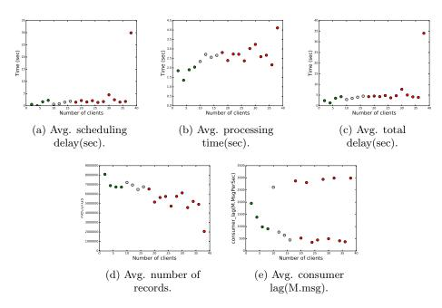
Figure 3.32 – Evolution of Spark software level metrics for setup-0 of the Kafka/Spark use case.
