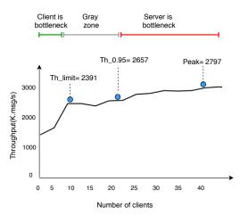
Figure 3.42 – Bottleneck identification for setup-0 in the full data processing pipeline.
