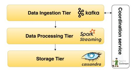
Figure 2.3 – Data processing pipeline
