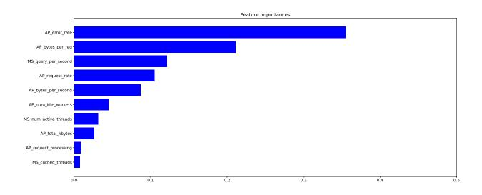
Figure 5.18 – Average importance of the proposed model features with the RF classifier for the LAMP stack.
