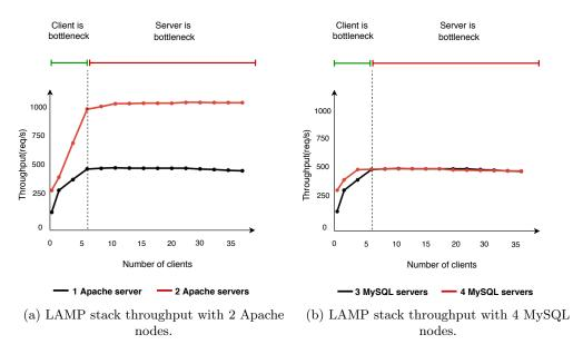
Figure 5.15 – LAMP stack throughput when provisioning more hardware resources.
