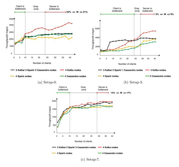
Figure 3.41 – Throughput(K.msg/s) of the full data processing pipeline for different setups and with different number of nodes allocated to each component.
