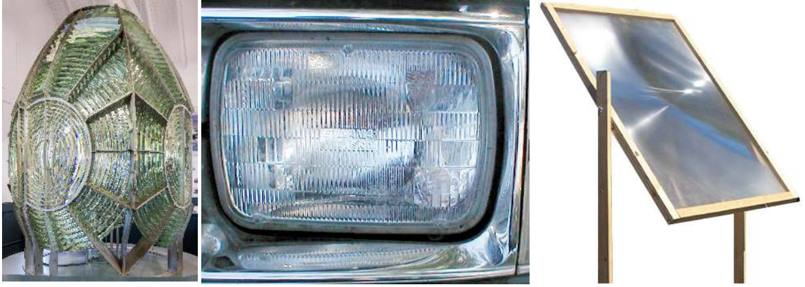
Figure 3.2: Example applications of Fresnel lenses. Left: Lighthouse. Center: Automobile headlight. Right: Solar concentrator
