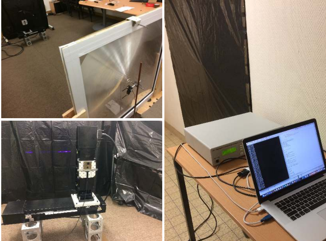
Figure 3.23: Pictures of the Fresnel lens localized diffusion experiment setup. Top left: A Fresnel lens is standing on the front and in the back is the XY scanner. Bottom left: A close up view of the XY scanner holding the photodiode, the black cover on the back shows the diffracted beam of the laser. Right: The door is carefully covered from outside, the instrument cables are passed through a door shaft carefully isolated from exterior light and the cables are connected to the motion controller and powermeter (not visible).
