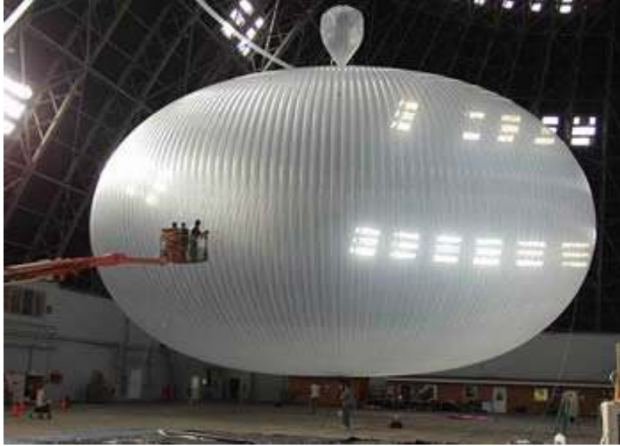
Figure 4.5: Fully inflated super pressure balloon, the vertical lines running from top to bottom of the balloon are the PBO tendons and the space delimited between each one is a gore.
