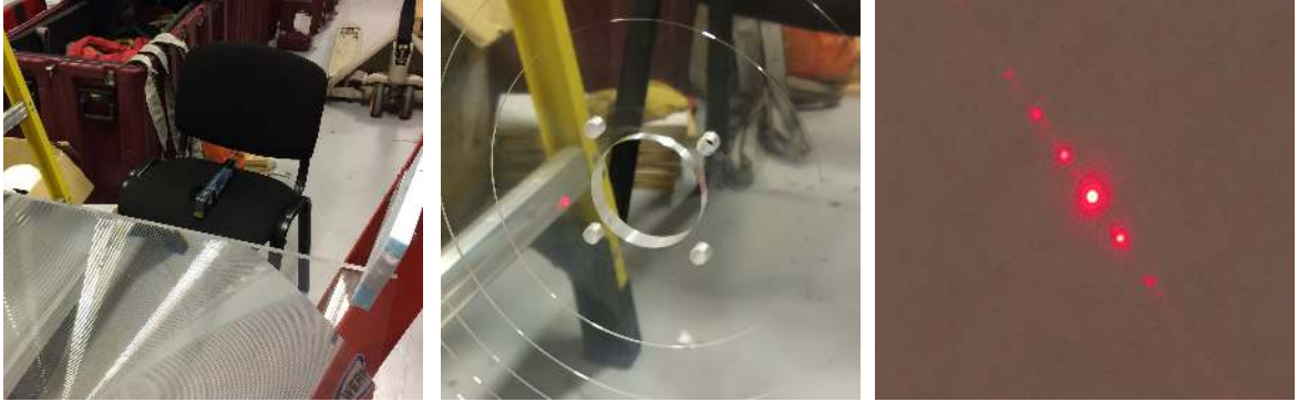
Figure 3.19: Improvised test to verify diffraction produced by individual Fresnel zones. Left: A red alignment laser used as pointer. Center: Laser dot visible on the first Fresnel zone. Right: The diffraction pattern produced when the laser beam goes through the lens.
