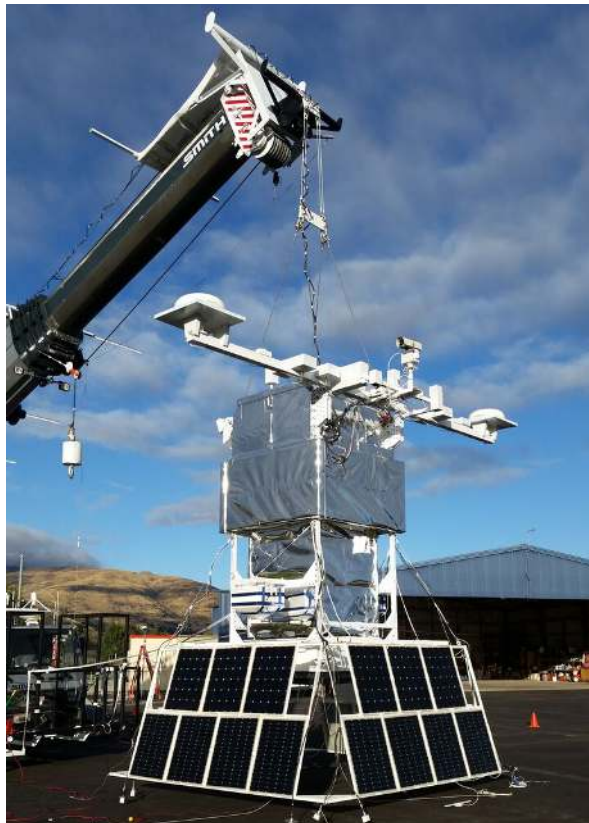
Figure 4.11: Hang test of EUSO-SPB1. The complete balloon payload (Instrument and Gondola) is integrated and hanged in order to be thoroughly tested and assess the launch readiness of the instrument.
