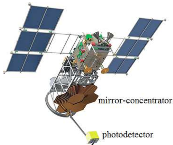
Figure 2.16: Schematic depiction of the Lomonosov satellite hosting the TUS detector. The mirror and photo detector module can be seen in front. Picture from [76].
