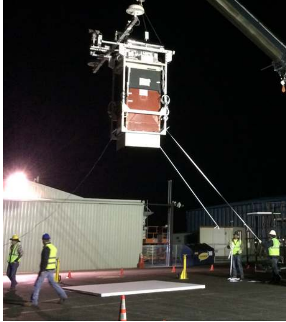
Figure 4.9: EUSO-SPB1 Flat fielding procedure at the Wanaka airport. The Tyvek screen is below the EUSO-SPB1 telescope pointing downwards.
