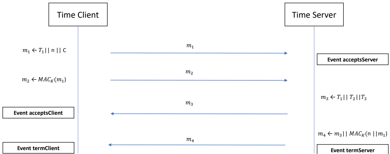
Figure 3.3 – Four events added in the protocol description in ProVerif to evaluate authentication and integrity properties
