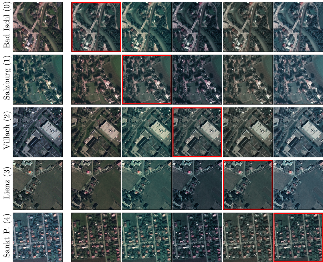
Figure 4.7: Real data used in the first experiment and the outputs generated by StandardGAN. Left column: the real data. Matrix on the right: The standardized data are highlighted by red bounding boxes. The rest of the cells depict the i^{th} domain with the style of j^{th} domain. The domain ids are indicated inside parentheses.
