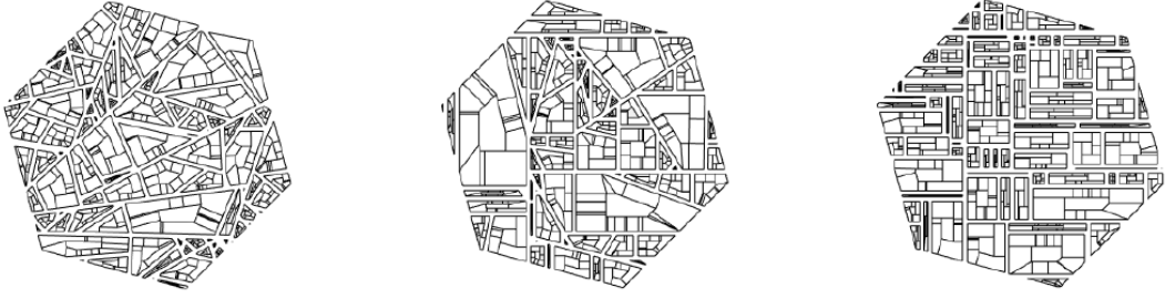
Figure 5.8: Footprint of three virtual cities with different anisotropy: from left to right, anisotropy values are: 0, 0.5 and 1 also called a Manhattan-like city.
