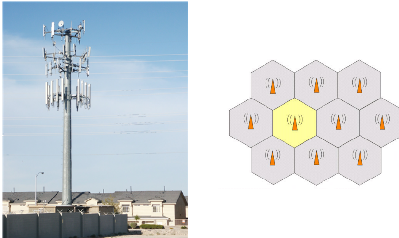
Figure 5.3: Cell phone base station antennas on a roof (left) - A small cellular network of uniform cell size (right).
