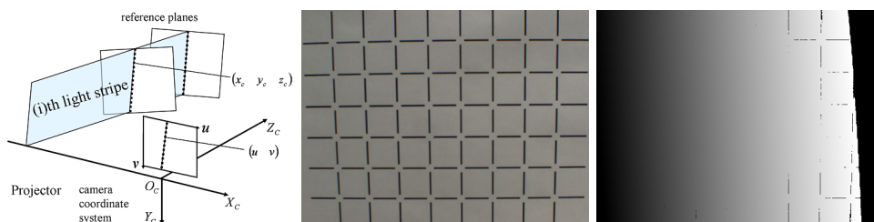
Figure 5.1: Projector’s light stripe calibration. Left: the setup of the calibration system. Middle: calibration board. Right: light stripe projected onto the calibration board. [Yamauchi 2008]
