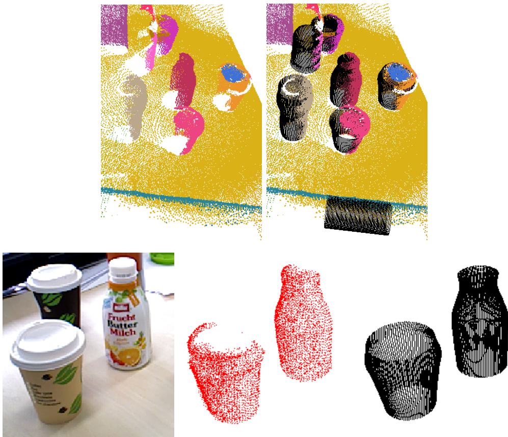
Figure 6.10: Dataset 2. Top: Original segmented point cloud (left) and our reconstruction result (right). Bottom: visual comparison between RGB image (left), original point cloud (middle) and reconstruction result (right) for Cup and Can objects.
