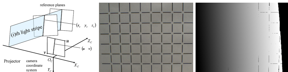
Figure 5.1: Projector’s light stripe calibration. Left: the setup of the calibration system. Middle: calibration board. Right: light stripe projected onto the calibration board. [Yamauchi 2008]
