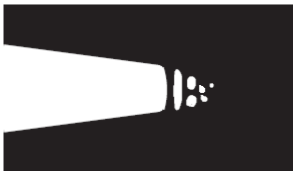
Figure I.4.3: Crack propagation in rubber-like materials involves cavity formation, chain pull-out and bond breaking [25].
