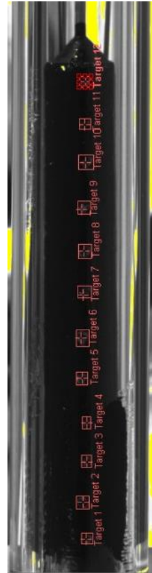
Figure III.3.3: Target Tracking using IMETRUM® Video Gauge™.
