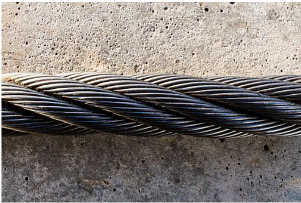
Figure V.1.1: Steel cord used in commercial car tyres
