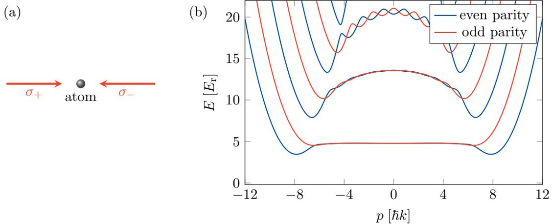
Figure 2.9: (a) Scheme of the laser configuration leading to a dynamics described by the Hamiltonian (2.2). (b) Dispersion relation calculated for the Hamiltonian (2.2) with  $\hbar\Omega = 0.35 E_r$  and  $q = 0.04 E_r$ . The even- and odd- $m$  sectors are uncoupled and represented in blue and red, respectively. The ground bands for each sector are almost degenerate in the bulk mode region  $|p| \lesssim J\hbar k$ , forming an effective band with Chern number  $\mathcal{C} = 2$ .
