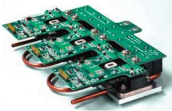
Figure 3.3: Cold plate for electronic cooling [9]
