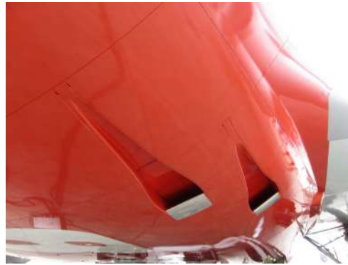
(a) RAM air intake example [35]
