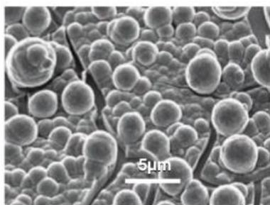
Figure 4.7: SEM image ( $30^\circ$  tilt) of the electrodeposited catalyst after  $30 C/cm^2$  were passed in  $0.1 M KPi$  electrolyte (at  $pH 7.0$ ) which contains  $0.5 mM$  of  $Co^{2+}$ .
