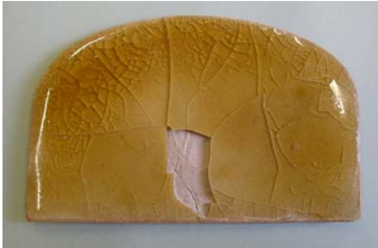
Figure 4.6: Sample of Simulated Ru Guan porcelain that fired according to the firing schedule (4.5)
