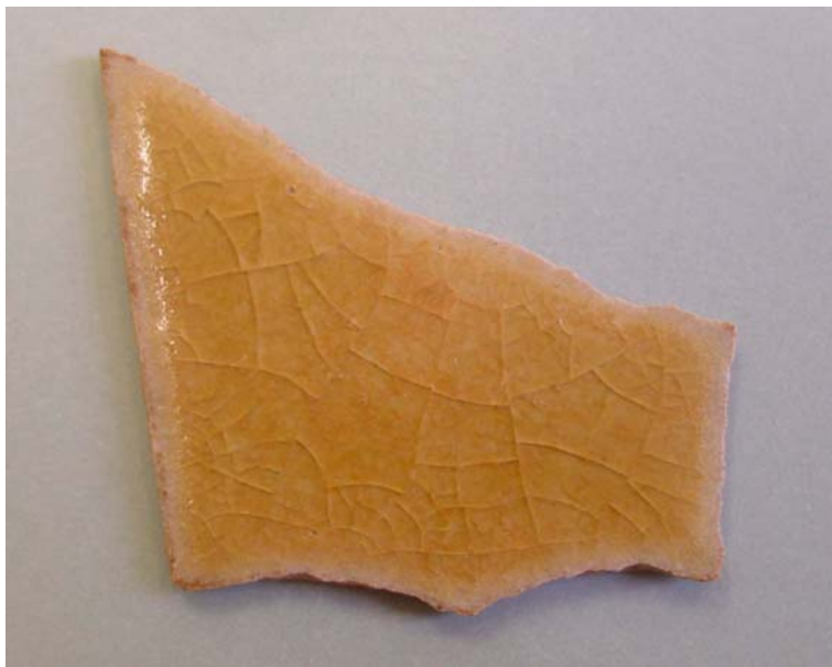
Figure 4.7: Successful simulated sample (R47) of Ru Guan porcelain with crackle treatment, according to calcined glaze recipe and firing schedule (4.5)
