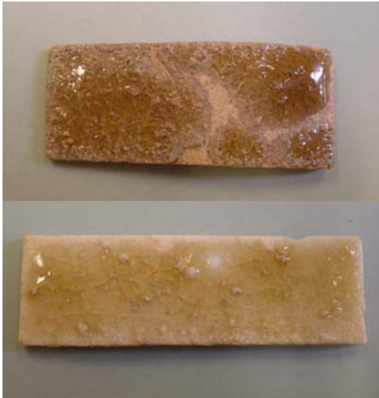
Figure 4.4: Apply the simulated glaze of R47G on the surface of simulated R47b porcelain body
