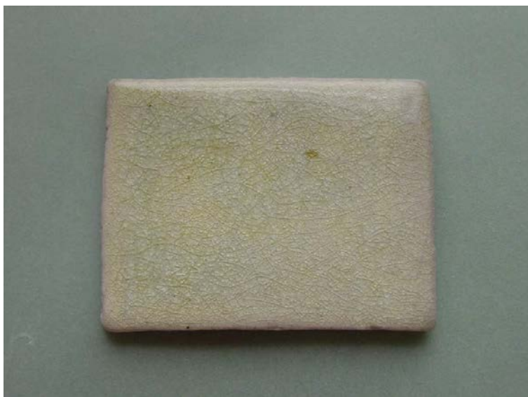
Figure 4.9: Esthetic treatment of crackle, created by thermal shock at 900°C.
