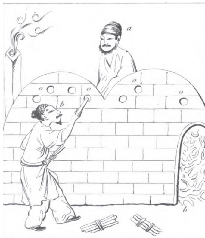
Figure 2.56: horizontal Chinese kiln constructs of two firing chamber
