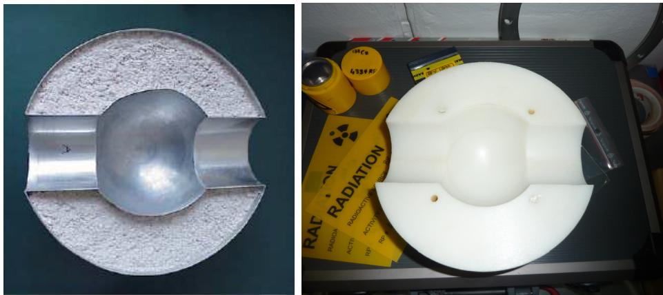
Figure 2.6: One hemisphere of the \text{C}_{12}\text{H}_{20}\text{O}_4(^6\text{Li}_2) neutron absorber used during the measurement of ^{234}\text{U} (left) and one hemisphere of the borated polyethylene neutron absorber used for ^{236,238}\text{U} (right).
