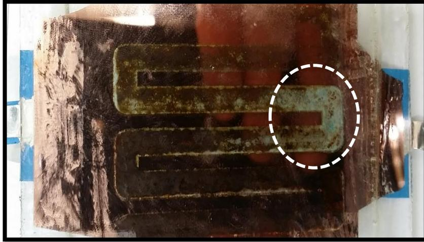
**Figure 3.1.** Typical oxidation of electrode (made with copper) in presence of oxygen.
