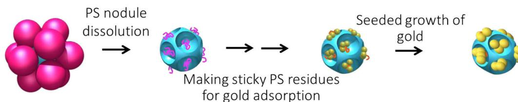
Figure 34 Synthesis schematization for the nanoparticles with patches [50]
