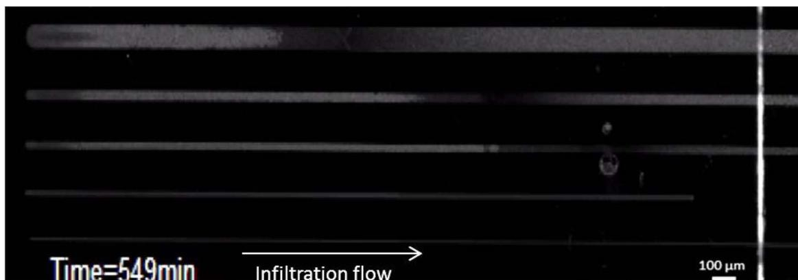
**Figure 77** Capture of the end of the infiltration experiment. The white part is the latex material assembled and the dark part represents the filling of the channels by PVP.
