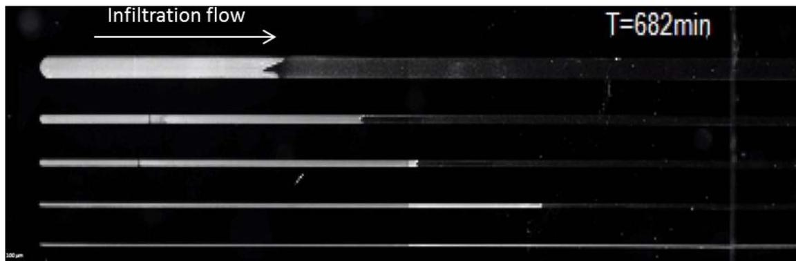
**Figure 73** Images acquired at the end of the experiments. All the channels are filled with the latex assembled particles (in white) and infiltrated with the PVA solution.
