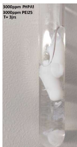
Figure 3.1 : Syneresis phenomenon observed after only 3 days for the gel sample prepared with a PHPA1/PEI25 ratio of 1/1.
